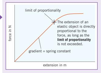
The spring constant can be calculated using the equation:
