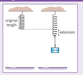
The **extension** is the increase in length of a stretched object from its original length.
