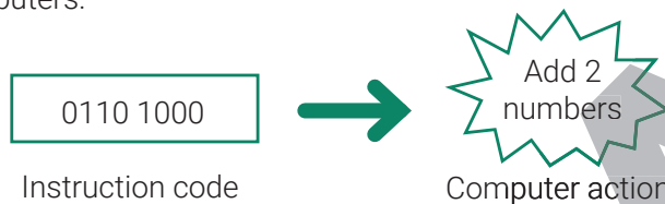
▲ Figure 8.1: A machine code instruction is decoded and executed
